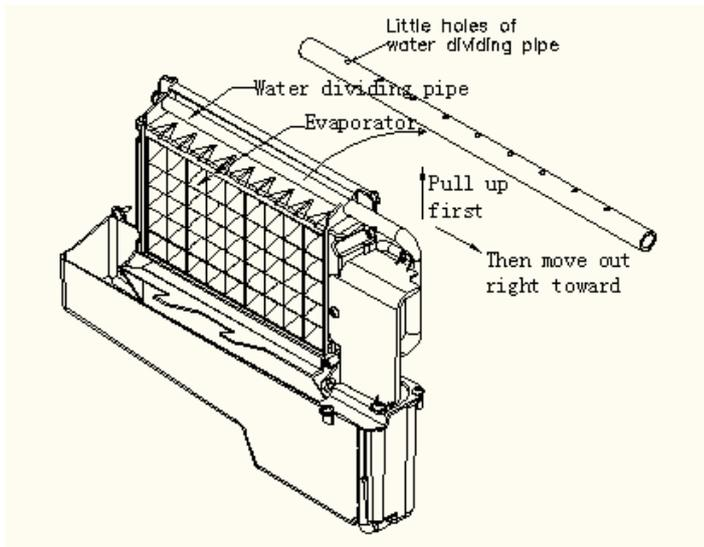
**4. For the water tank and ice-full detecting plate**
