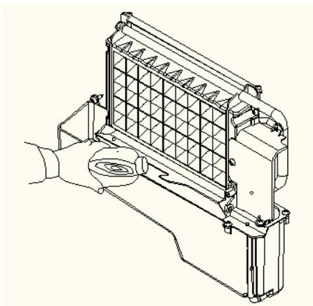
5. Turn on the power to the ice maker, then press “TIMER CLEAN” button on control panel for more than 5 seconds, to enter the self-Cleaning program. Same as above explanation, the water pump runs for 8 minutes and stops for 3 minutes, one cycle, again one cycle. The total duration time is 30 minutes for one self-cleaning program.
