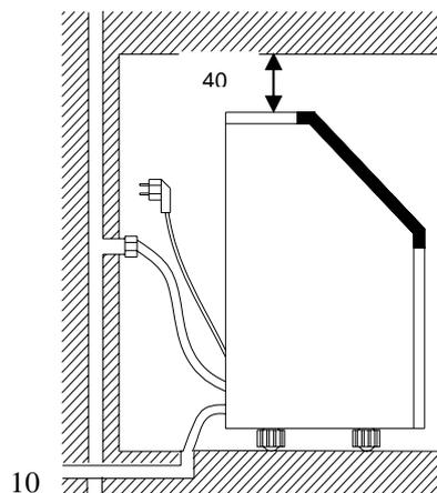
To ensure proper ventilation for your ice maker, the front of the unit must be completely unobstructed (at least 20CM free space). Allow at least 150 mm clearance at rear, and 50 mm at top and sides for proper air circulation. The installation should allow the ice maker to be pulled forward for servicing if necessary.
