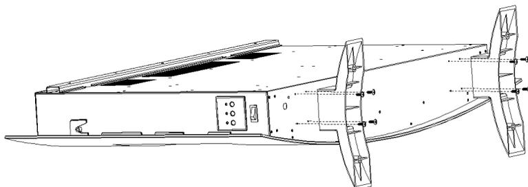
Fix the standing leg on the products by using the 4\*16mm screws, as shown in the figure above.
